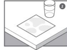
Place a dampened sheet of kitchen roll over the area where the micro-scratches can be seen.
